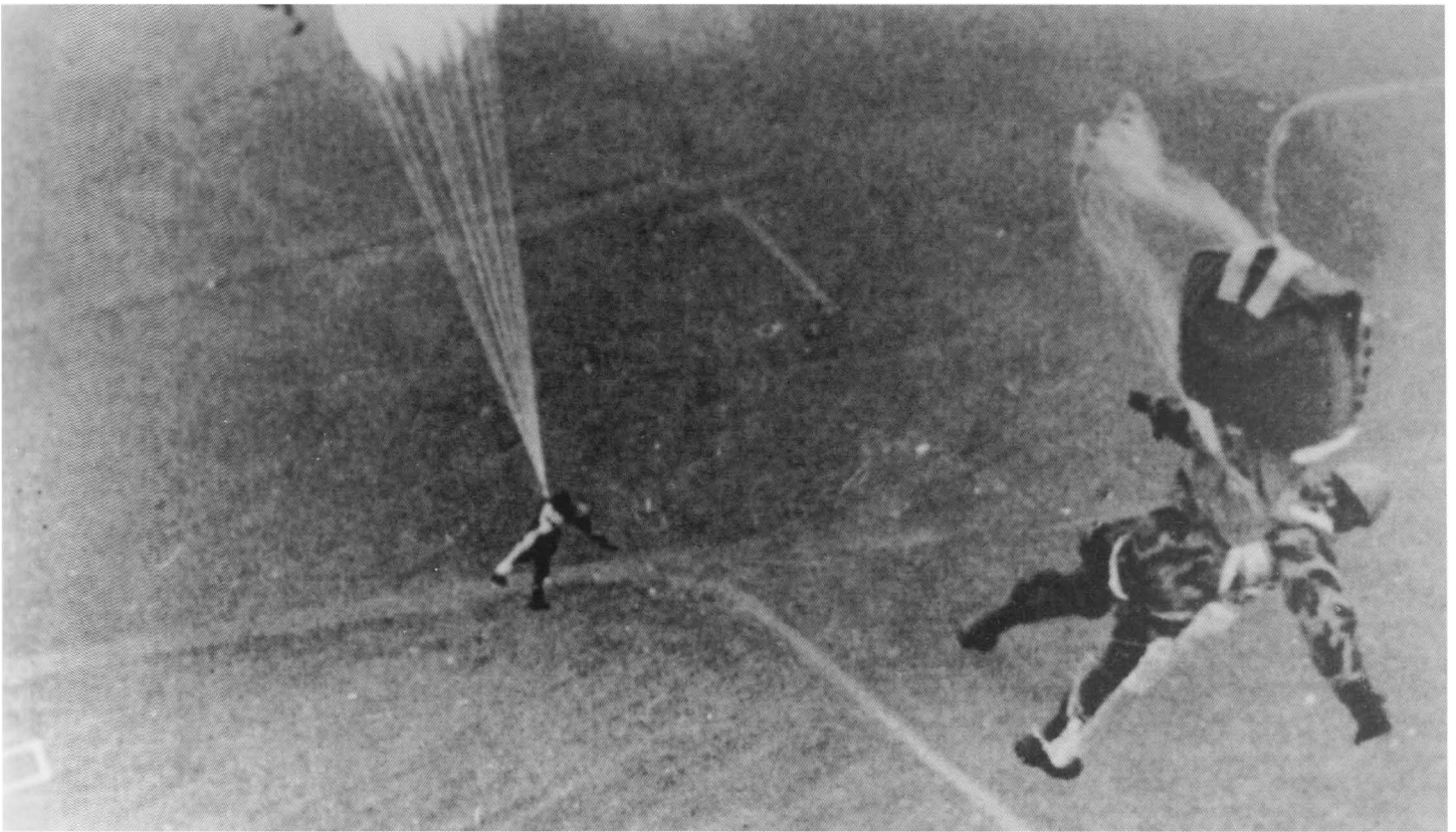
The IF 41 SP being jumped. The suspension lines being pulled from the bag are bowed in the slipstream as is the static line.
