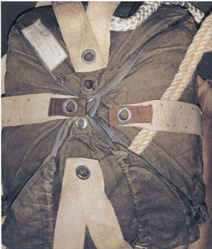
Closing arrangement for bag and straps on the RZ 36. Pull up cord in top photo shows routing.
