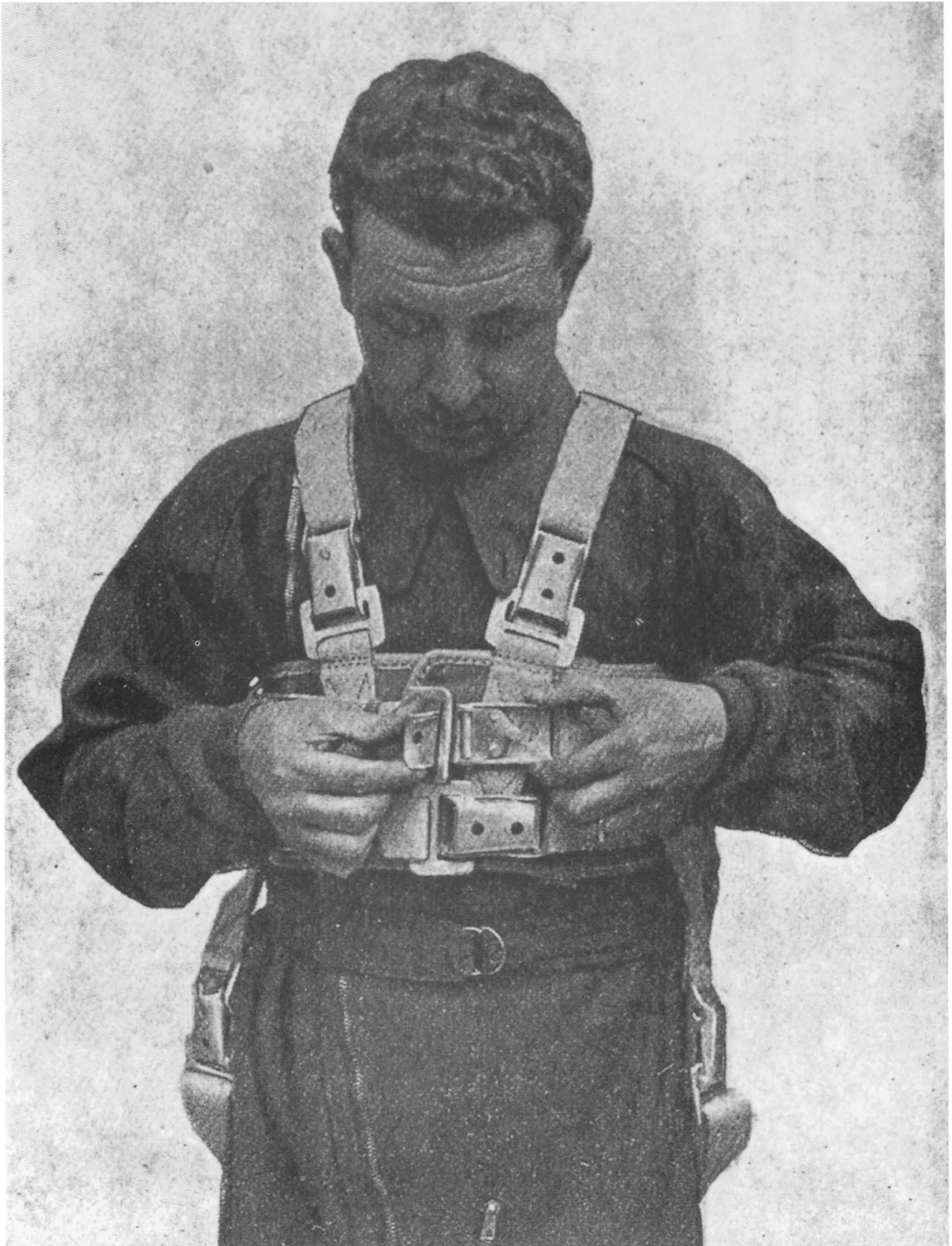
Demonstration of the closure of the chest straps by means of the quick ejection/locking system.
