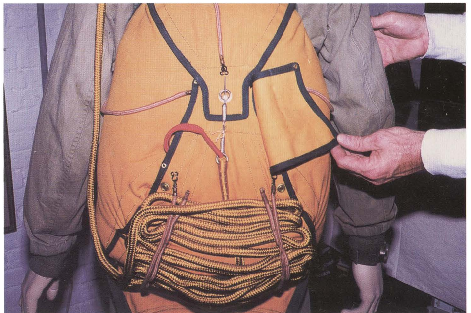
The army main parachute stowed the static line on the bottom of the pack tray under two flaps. The main canopy was not bag deployed, unlike the Navy rig, but the container was closed in a similar manner.
