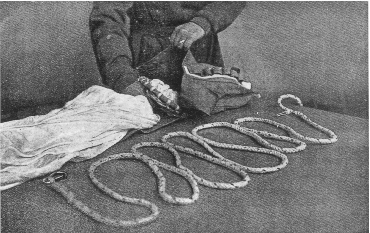
16.) Place the silk chute into the sack starting from the rubber ring opening . . .
