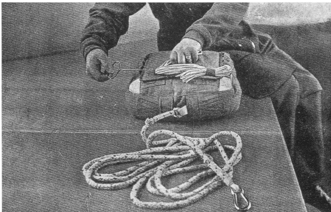
19.) Close the sack and place the ropes as shown in the photo beneath the sack cover.
