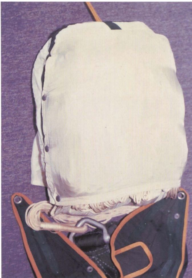
Top of deployment bag showing static line attachment.
