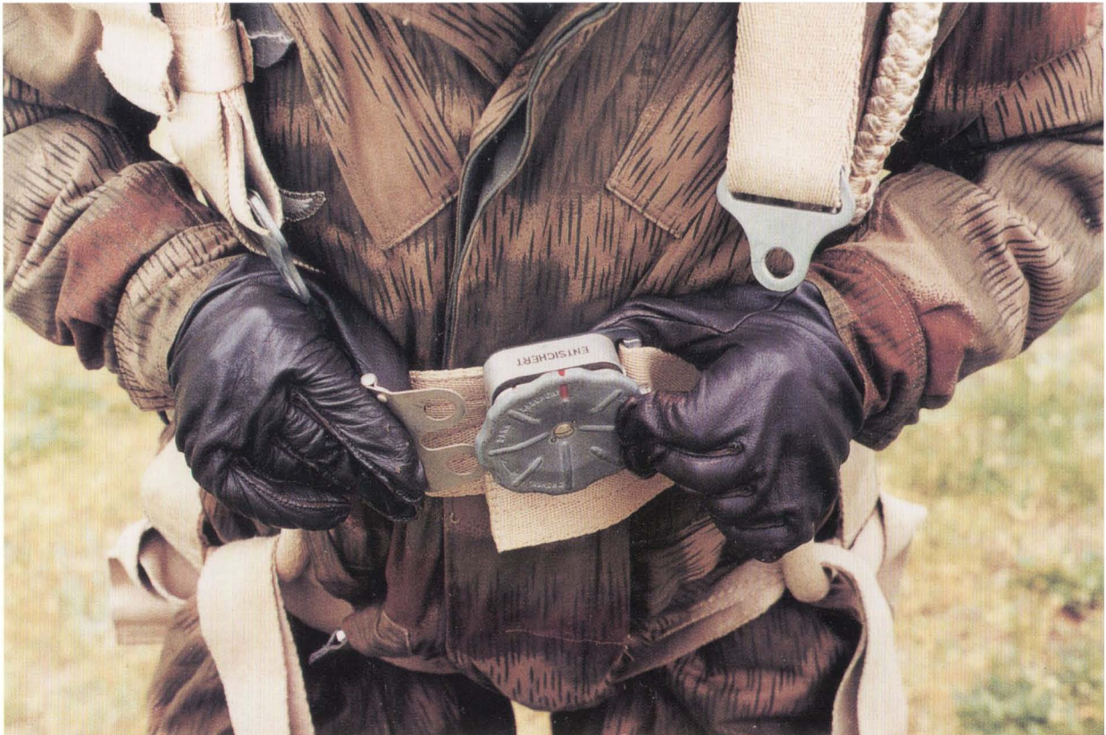
Single point quick release with locking fork.
