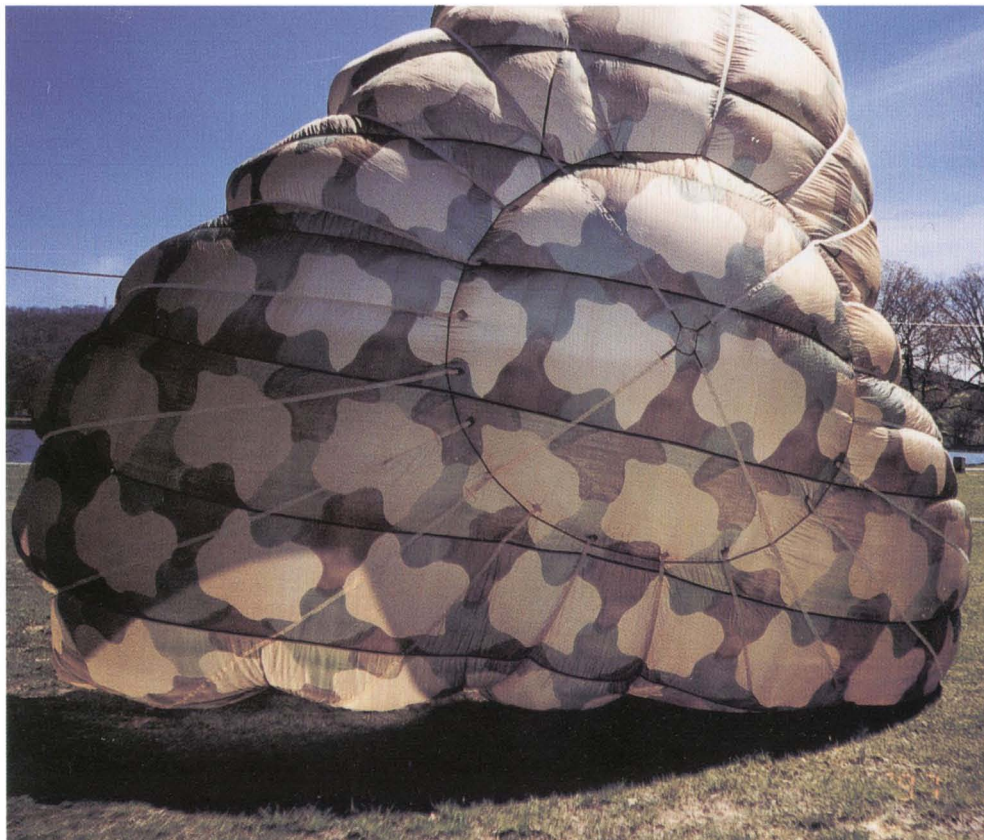
The RZ 36 canopy was delta shaped with a flat leading edge and the V-tail providing a vent thereby reducing oscillation.
