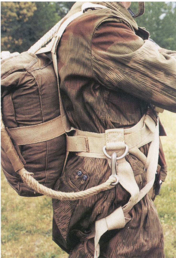
The RZ 36 harness suspended the jumper in the same manner as the earlier systems.
