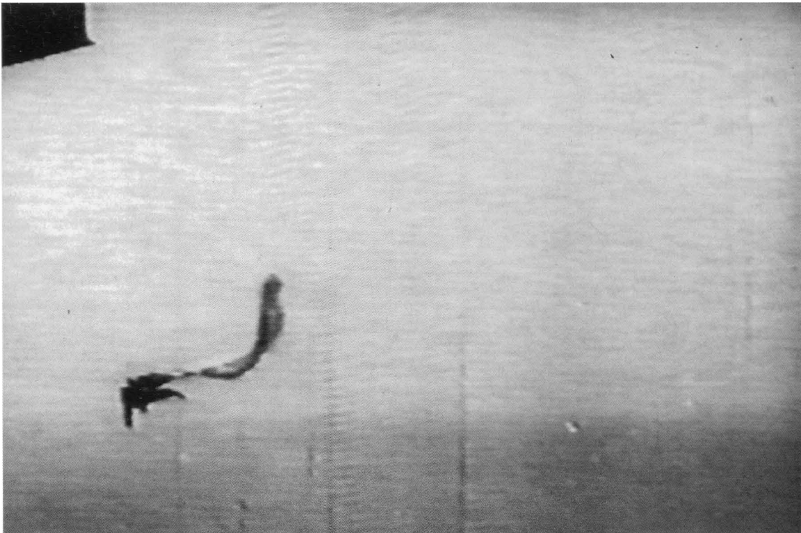
The static line has pulled the canopy peak out into the slipstream.
