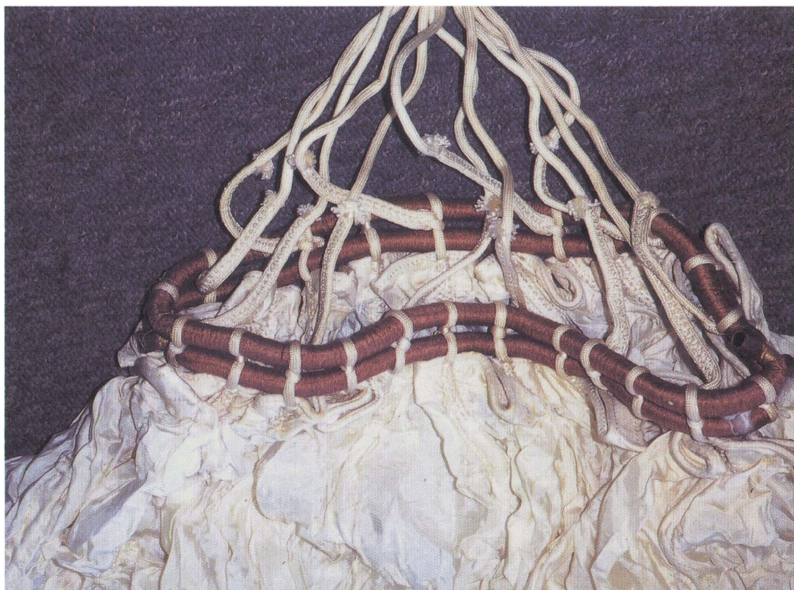
Static line apex tie.
