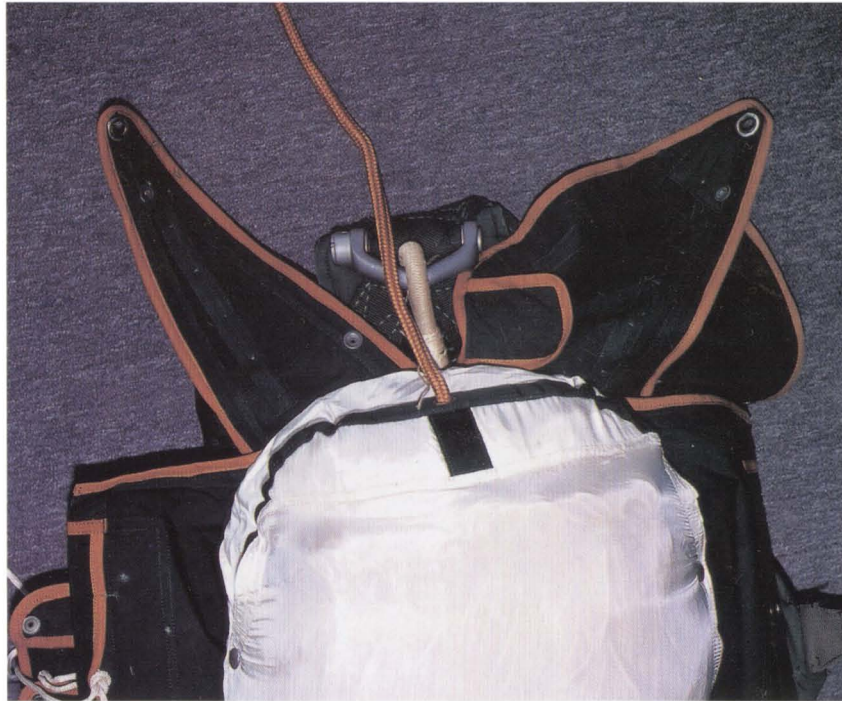
Top of deployment bag showing static line attachment.
