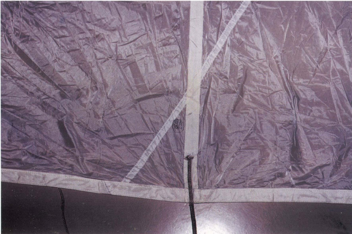
Suspension line attachment to RZ 36 at radial seam.
