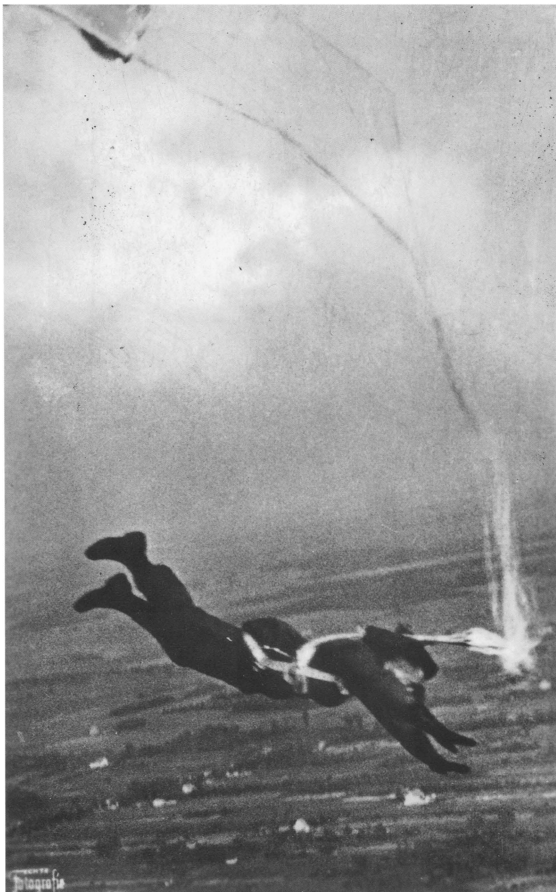
The RZ 1 lines were drawn from the deployment bag in an abrupt manner – loose in the slipstream. Here the container, retained by the risers, has blown up behind the jumper's neck.
