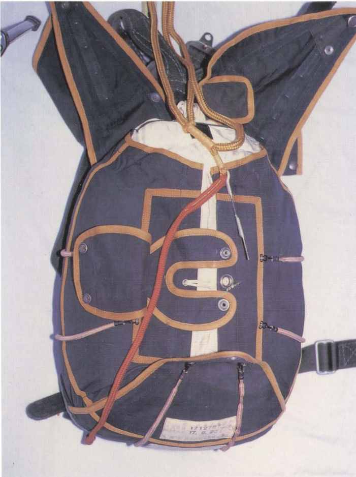
Naval troop parachute container closure.
