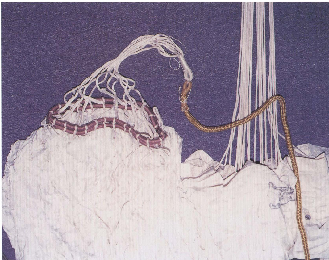
Static line apex tie.
