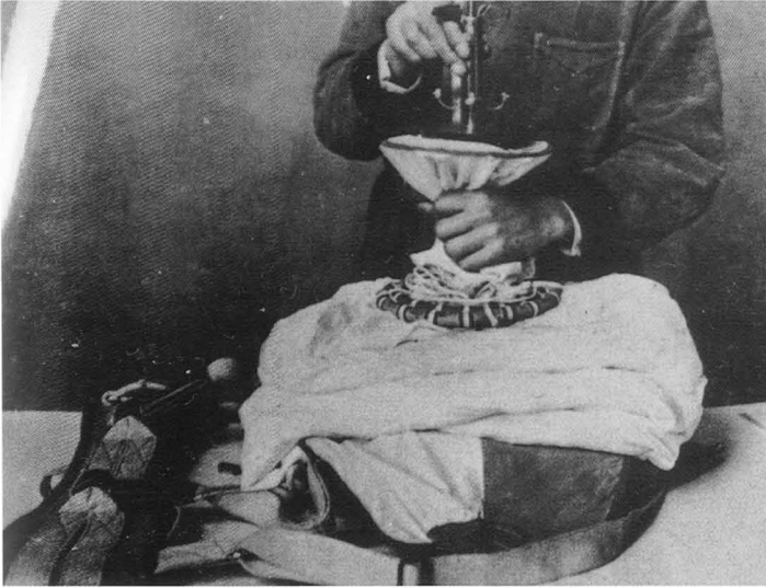
The winding key is applied to the pilot parachute.
