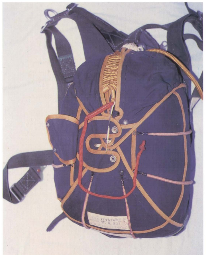
Container closed, locked with pin. Static line stowed.
