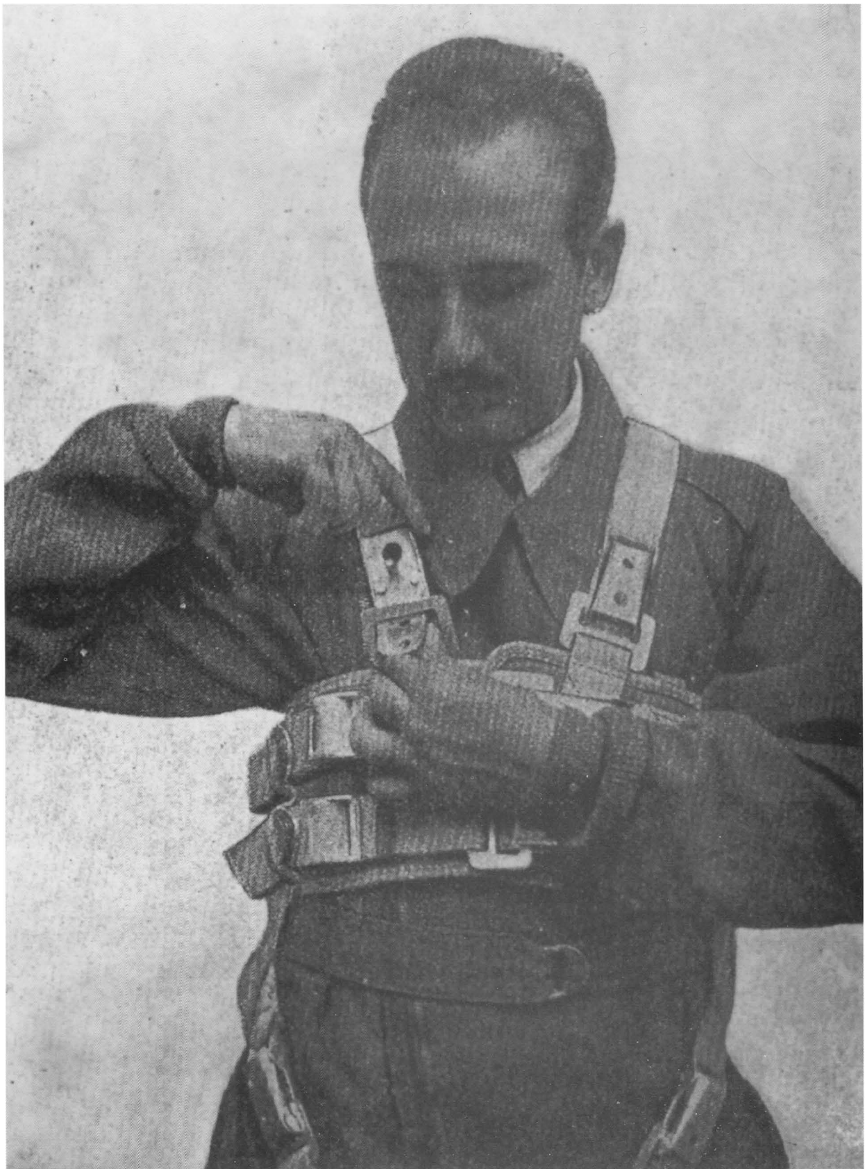
Demonstration of the closure of the shoulder and thigh straps. The parachutist adjusts the shoulder and thigh straps to assure that they are snug. The adjustment eliminates the possibility of the parachute being too tight or too loose.
