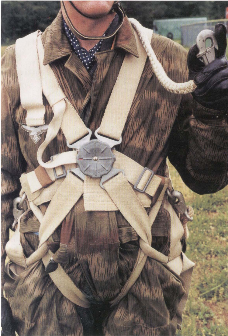
Quick release button in the secured position.
